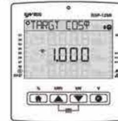
Enter the reference step and press OK. (Reference level must be 3-phase capacitor.)
