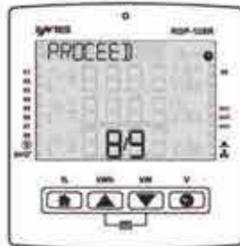
The OK icon will light up on the upper right corner of your device. With the 'Enter Details' option, you can access the content of menus or confirm the settings you want to store. Press OK.
