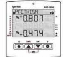
Press and hold the UP direction key for 2 seconds to go to the active import energy.
