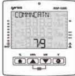
The OK icon will be enabled on the upper right corner of your device. You can use the Up and Down direction keys to switch between main menus and sub-menus. Press OK.
