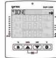
Your Power Factor Controller has started to recognise the steps automatically.
